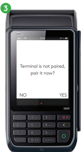
**Power on the terminal.** If the terminal has not been paired previously it will display "terminal is not paired, pair it now?" If you do not see this screen, refer to the full integration guide at [smartpay.co.nz/guides](http://smartpay.co.nz/guides) for instructions.
